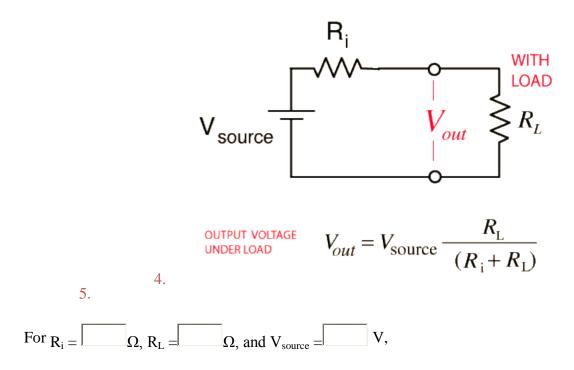
The open circuit output voltage would be equal to  $V_{source}$ , but when it is connected to the load, the output voltage will drop to  $V_{out} = \Box V$ .
