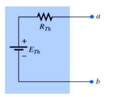
Procedure to determine the proper values of  $R_{Th}$  and  $E_{th}$ :
