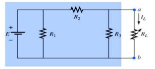
2. Mark the terminals of the remaining two-terminal network. (The importance of this step will become obvious as we progress through some complex networks.)
