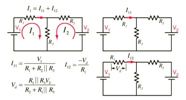
$R_1 || \; R_3 \;$  means the parallel resistance of  $R_{\scriptscriptstyle J}$  and  $R_{\scriptscriptstyle S}$  .
