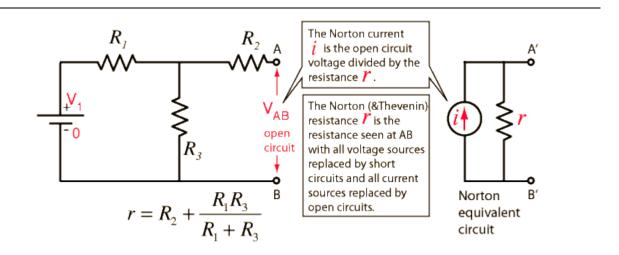
NUMERICAL EXAMPLE APPLIED TO TWO LOOP CIRCUIT :
